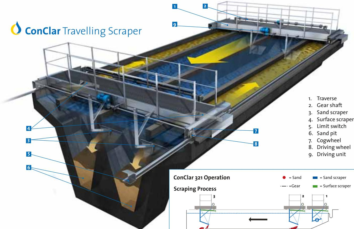
ConClar 321/325 is a travelling bridge scraper for rectangular grit chambers which can be delivered in two performances:
